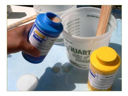
Pour the mold material – it is important that you pour the rubber material in the lowest spot of the container, and NOT directly on the model. This is to prevent trapping air bubbles on your model.
